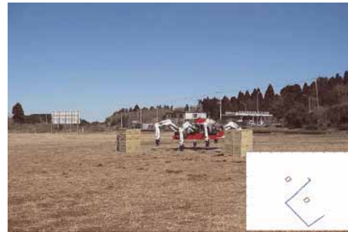
Figure 6. Photo of the obstacle avoidance test by tele-operation
