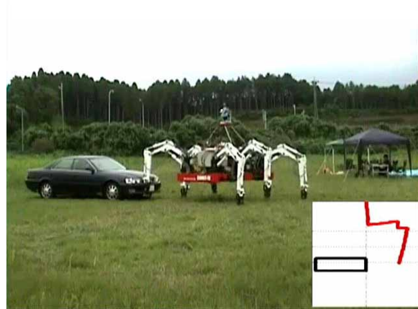
Figure 4. Photo of the obstacle avoidance navigation test
