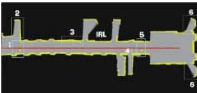
Fig. 4. Mapping using the laser scanner. The marks 1 to 6 are problematic cases for the scanner.
