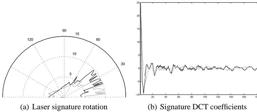
Figure 8: DCT based spectral analysis under phase shift (rotation)
