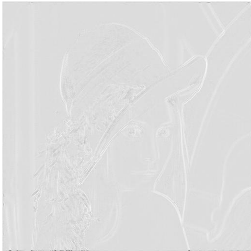
Figure 5. The negated normalized difference between two implementations of Canny's detector. One uses derivatives without smoothing to compute the gradient and the other one uses Sobel's operator to compute the gradient.
