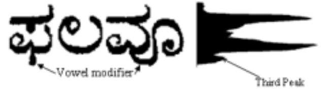
Figure 15: A sample word having characters with their vowel modifier extended to bottom zone and its Horizontal Projection Profile
